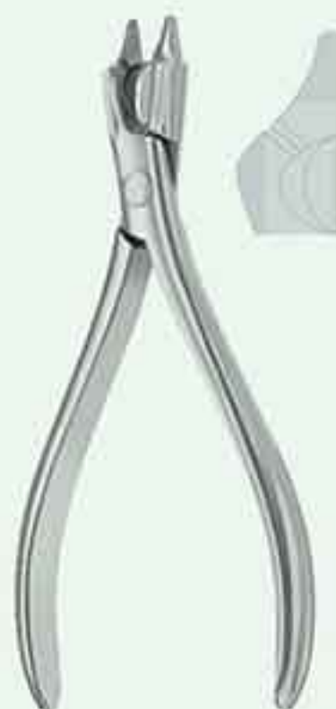
Universal 48-185-15 15.5 cm - 6" 48-186-17 17.5 cm - 6¾" Bends: hard wire upto 0.9 mm / .035" Ø max. Cuts: hard wire upto 0.7 mm / .028" Ø max.
